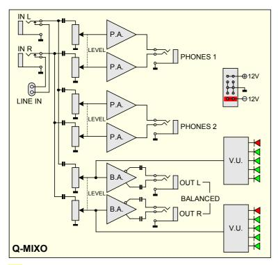
**NB:** The rear wiring from the Q-MIX is automatically cut off if you insert a source into the input jacks.
