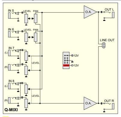
**NB:** if you only have a mono signal for stereo inputs 7 and 8, use the left input, it will automatically be connected to the right input.
